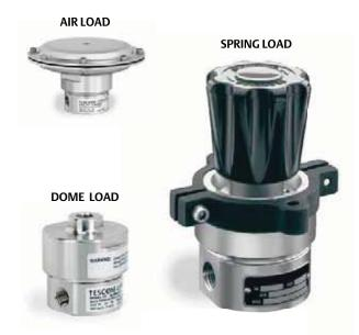
TESCOM 26-2300 Series is a highly accurate, diaphragm sensed backpressure regulator. It controls pressures up to 500 psig / 34.5 bar and offers many  $C_V$ s from 0.02 up to 1.0. Air and dome loaded versions are available for remote operation or for use with the TESCOM ER3000 Electropneumatic Controller for automation.
